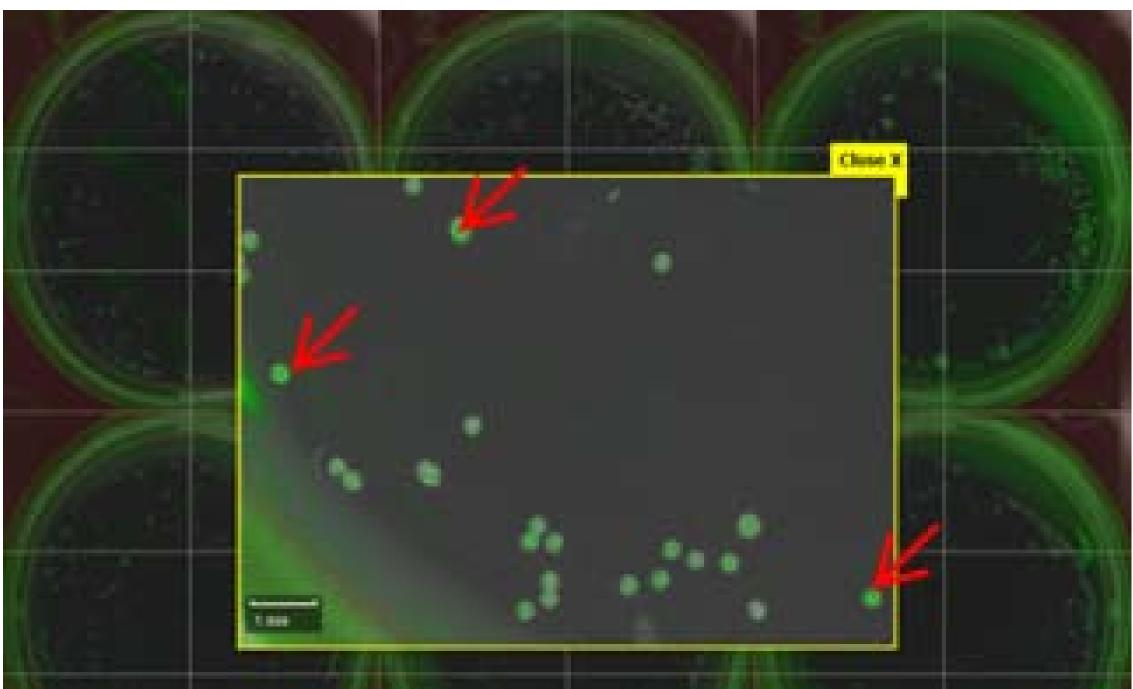
Figure 4: Composite image (White Light image with FITC overlay) of the stem cell coated beads on ClonePixTM. The zoomed in image identifies three beads to be picked (outlined in green with red arrows) that meet the specified shape, size and fluorescence criteria amongst discarded beads (no outline displayed)
